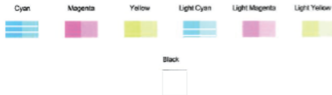
Figure 9-2 Example of color blocks with defects
